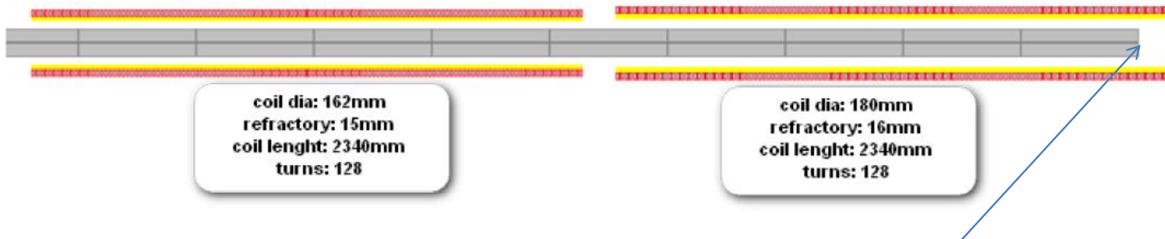
Figure 4. View of investigated induction system in 2DELTA program (100mm displacement)
